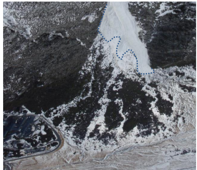
Figure 6: Avalanche in the Kitchener path, 24 July, 2009. Dashed blue line delineates approximate toe of deposit which overtopped the diversion berm (DOC photo).
