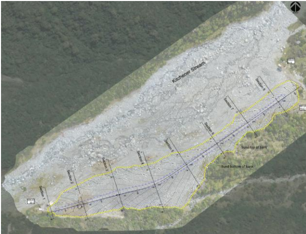
Figure 8: As-built diversion berm in plan view.
